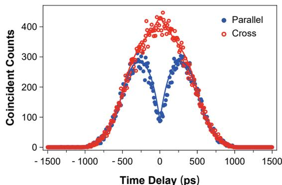
Left: Artist's interpretation of setup for two-photon interference between photons from a quantum dot (QD) and sunlight. The InAs/GaAs QD was embedded in a 2- $\mu\text{m}$  micropillar and sandwiched between 25.5 (15)  $\lambda/4$ -thick ALAs/GaAs mirror pairs, forming lower and upper distributed Bragg reflectors. Right: Two-photon coincidence counts at orthogonal (red) and parallel (blue) polarizations.
