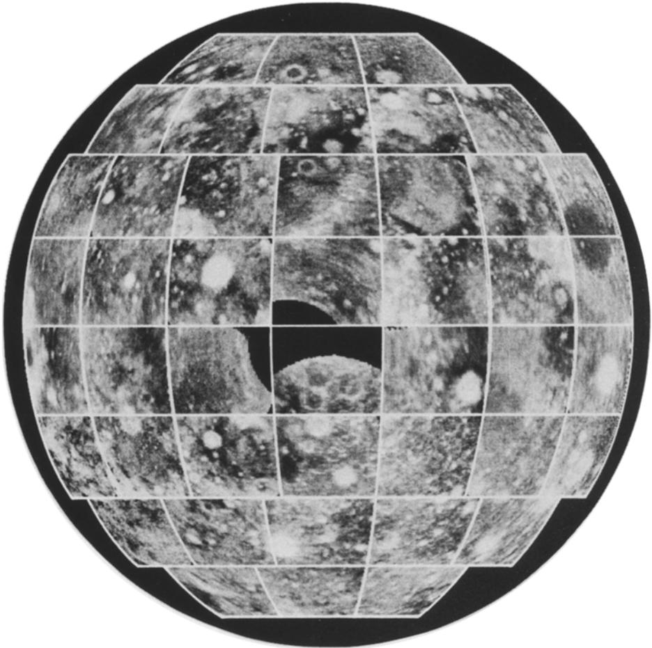
Fig. 5. A mosaic of depolarized lunar radar maps at 70-cm wavelength. The Moon is shown at mean libration and individual maps (corresponding to LAC Charts) are outlined. Radar echoes are normalized to show departures from the average; resolution is 5–10 km. See Figures 6, 7 and 8 for comparison with Earth-based optical and infrared observations.
